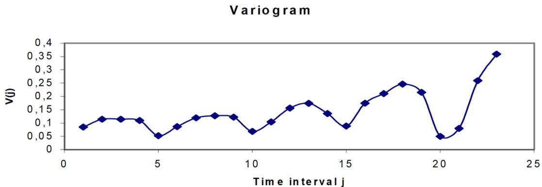
**Figure 9 Variogram for the time series in Figure 8. On the x-axis are given the different time intervals,  $j$ , used to calculate the variances,  $V(j)$  on the y-axis**
