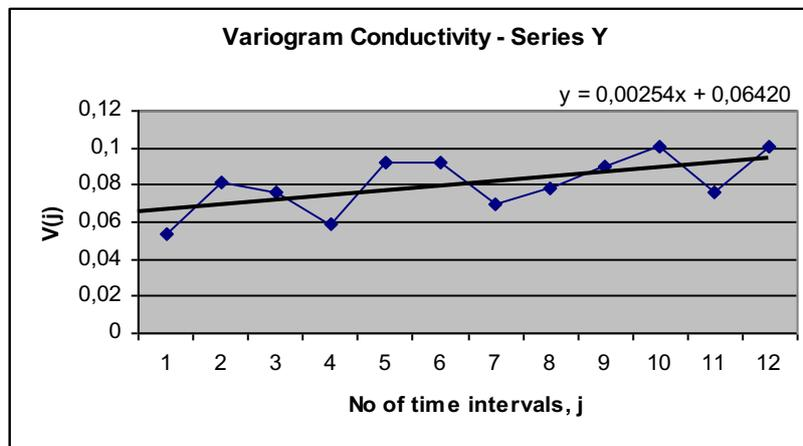
Figure D 6 Variogram of time series Y (2.5 minutes increments)
