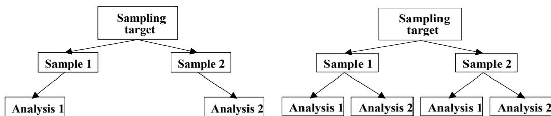
**Figure 5 The principles of the replicate design with (left) single split and (right) balanced double split (two level nested design)**
