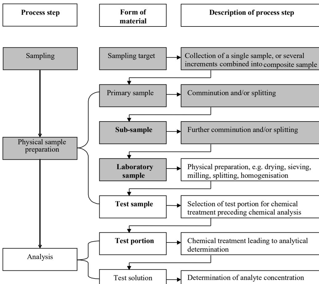
**Figure 1 Schematic diagram of a typical measurement process including sampling, physical sample preparation (including transport) and analysis**
