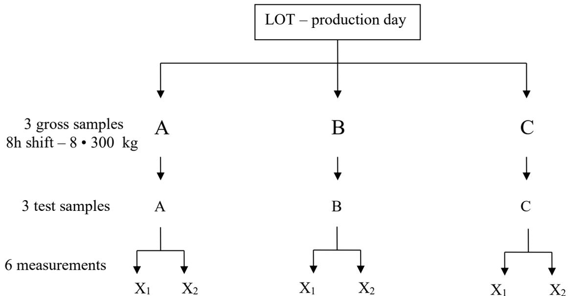
**Figure B 3 Experimental design, modified method 1 of ISO 3085, separating the primary sample into three shift samples (240 g) and splitting to a test sample (150 g) , duplicate measurements of each test sample**
