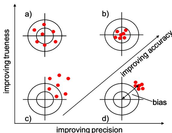
**Figure 4 The ‘shots’ on the target represent individual measurement results; the reference value is the centre of the target, courtesy of Eurachem [35]**
