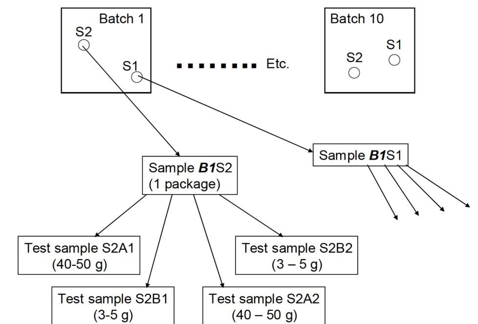
**Figure C 3 Splitting of the primary sample to make 4 test samples**
