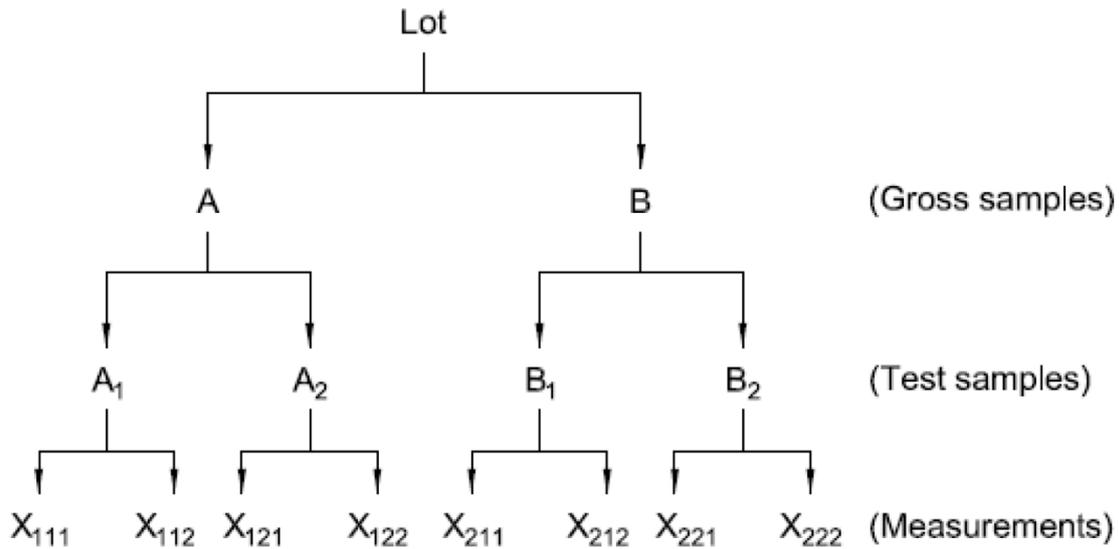
**Figure B 2 Experimental design using duplicates – ISO 3085 (1986) Method 1**
