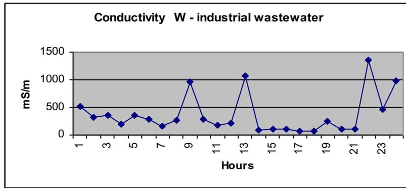
Figure D 1 Time series W (1 hour increments) – Conductivity
