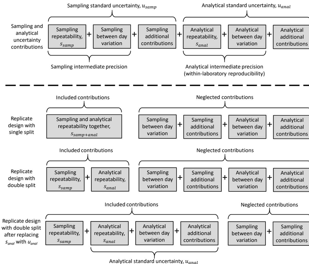
**Figure 6 Illustration of the uncertainty contributions that are included using the replicate design with a single split at the sampling step, or a double split – split at the sampling step and split at the analytical step**
