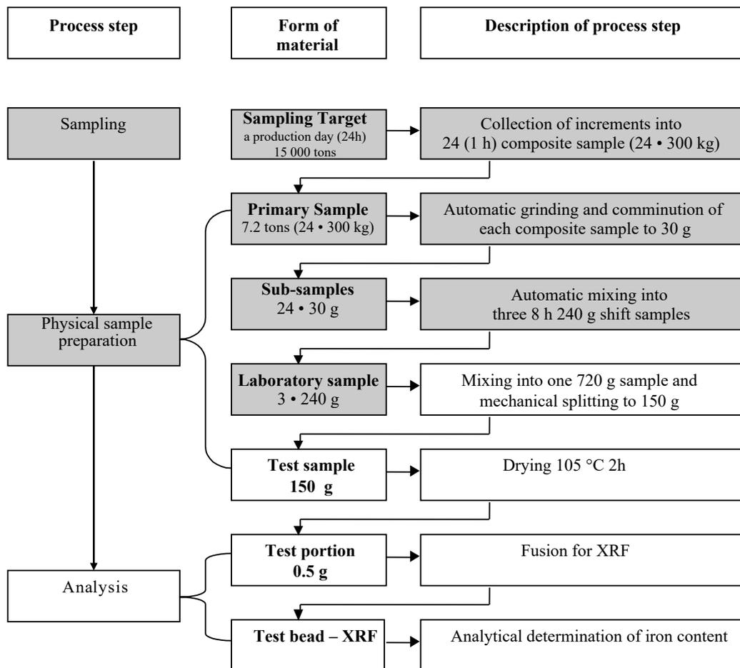
Figure B 1 Schematic diagram of iron ore sampling and analysis at LKAB, Kiruna
