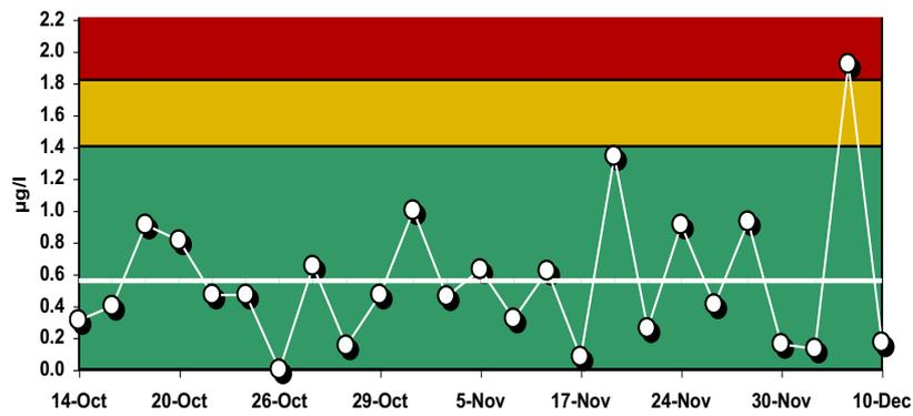
**Figure 7 Example of a range control chart for quality control of measurement (sampling & analysis)**
