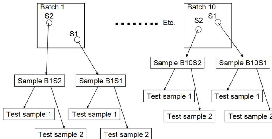
**Figure C 1 Sampling for validation. Two samples are taken from each of ten production units/batches of the same type of sample**
